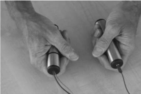
The segmented handhold must be placed in the right hand such, that the forefinger curls around the DIRP sensor without pressure. Both hands should be kept as steady as possible during the DIRP run to avoid false readings.
