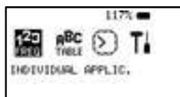
If the battery is fully charged its icon in the upper right corner of the display will show a load of more than 115% (117% ■). The battery icon flashes if the device is connected with the USB-cable to either the power supply or a booted PC or Notebook until the battery is fully charged.
