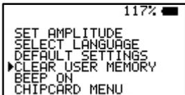
5. Now press [3] and keep it pressed. Press CENTER for half a second. When device beeps, release keys. Display shows activity and returns to main menu.
