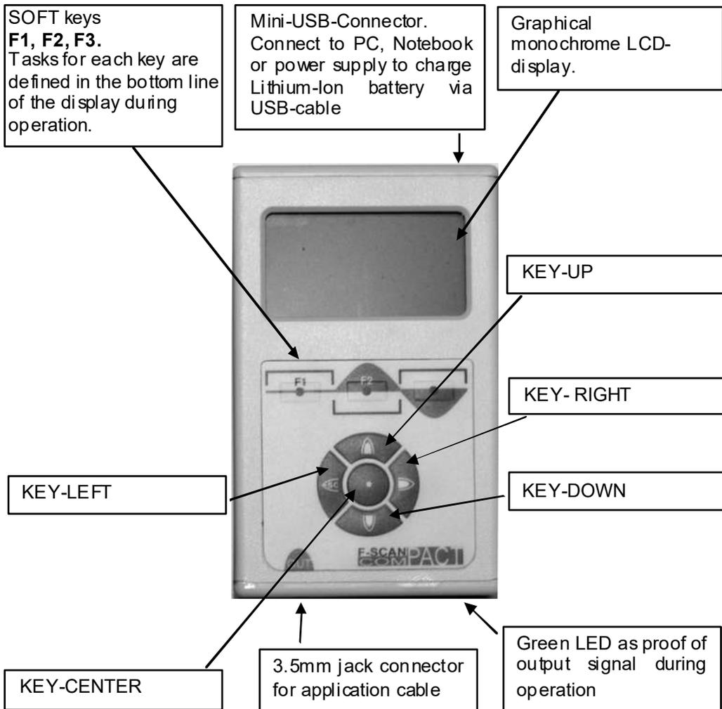
**NOTE:** The display lights up for a few seconds only to support input activities. The device switches OFF if inactivity exceeds 2 minutes. Both measures reduce the power drain on the battery.
