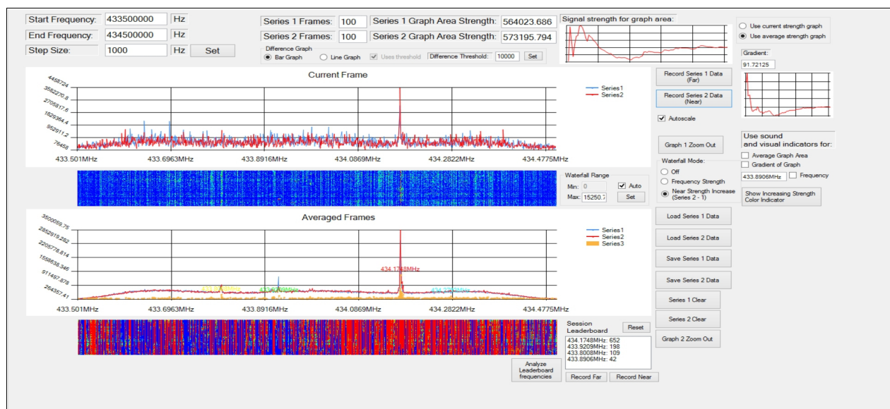
Figure 2-2 RTL SDR Reradiated Energy Detection System
