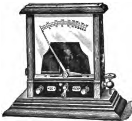
FIG. 31.—VERTICAL FORM OF MILLIAMMETER.
