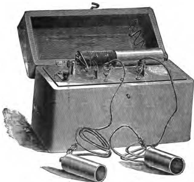
FIG. 104.—INDUCTION COIL WITH EXTERNAL DAMPING TUBE.
