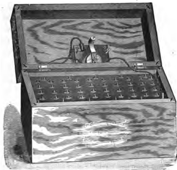
FIG. 20.—SILVER-CHLORIDE BATTERY OF FIFTY CELLS.
