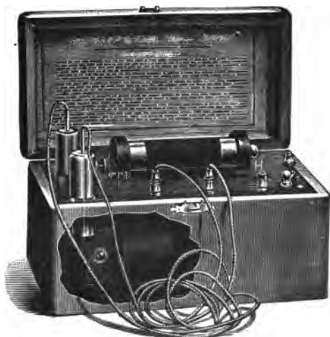
FIG. 103.—INDUCTION COIL WITH DRY CELL AND INTERNAL DAMPING TUBE.
