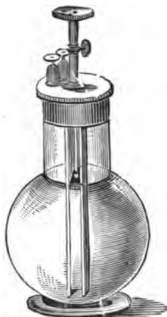
FIG. 12.—GRENET PLUNGE CELL.
