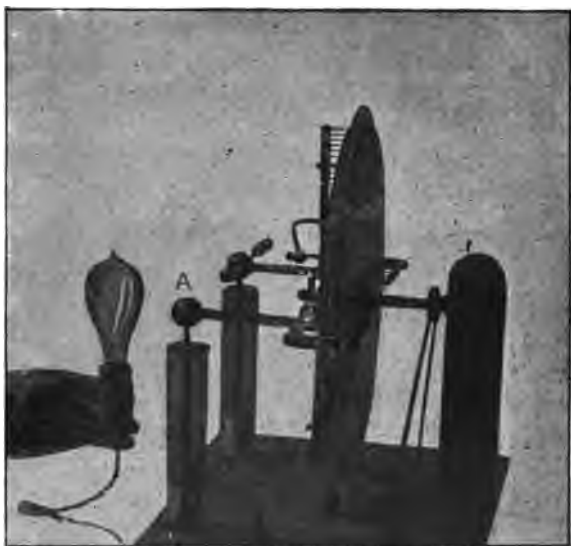
FIG. 4.—TRANSMISSION OF ELECTROSTATIC FORCE ACROSS A VACUUM.
