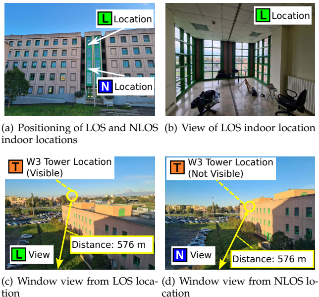
Fig. 11. LOS and NLOS indoor measurement locations.
