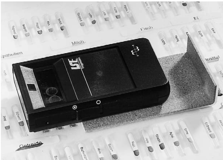
Fig. 6.4 Sender apparatus of the ISE system, to be used in conjunction with an allergen test set. A slider (plastic with cork coating) is used to test individual ampoules or ampoule groups. Only the ampoules not covered by the slider are registered.
