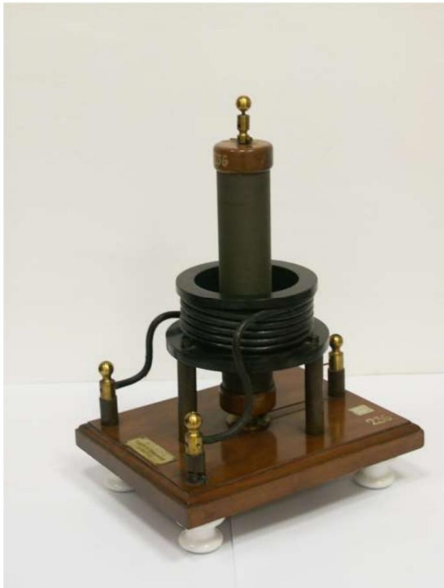
demonstration-educational Tesla transformer (without iron core)
