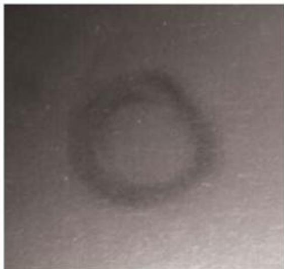
**Fig. 13.6** Microscopic view of droplet dissolution. A ten-microliter droplet of water was released onto water containing 1- $\mu\text{m}$  carboxylate microspheres. A ring-like clear zone implies an EZ sheath surrounding the droplet.
