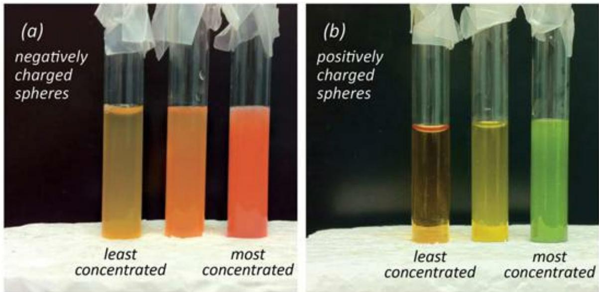
**Fig. 5.5** Addition of microspheres alters water's pH. (a) Carboxylate microspheres, 1  $\mu\text{m}$  diameter. Increasing microsphere concentration changes dye color toward red, indicating lower pH. (b) Positively charged amino microspheres change dye color toward green, indicating higher pH.
