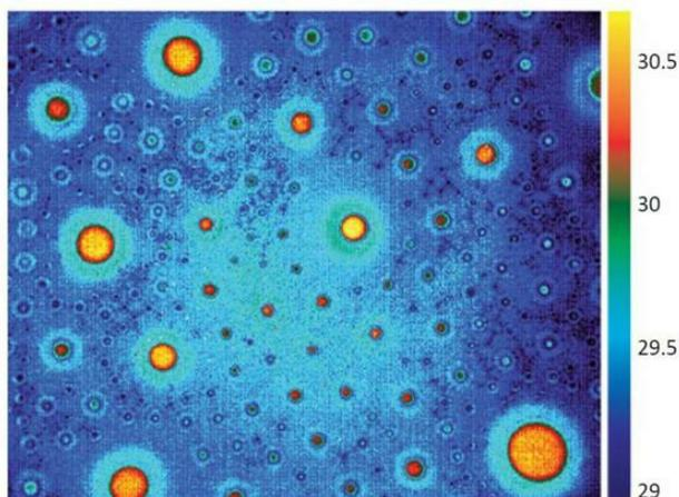
**Fig. 14.6** *Infrared image of surface bubbles. Bubbles were created by blowing air into a surfactant solution (TWEEN 20/water). Bubble interior (orange) generates more infrared energy than the exterior (blue). Darkness of thin bubble boundaries is expected — EZs generate little infrared energy. Scale in °C.*
