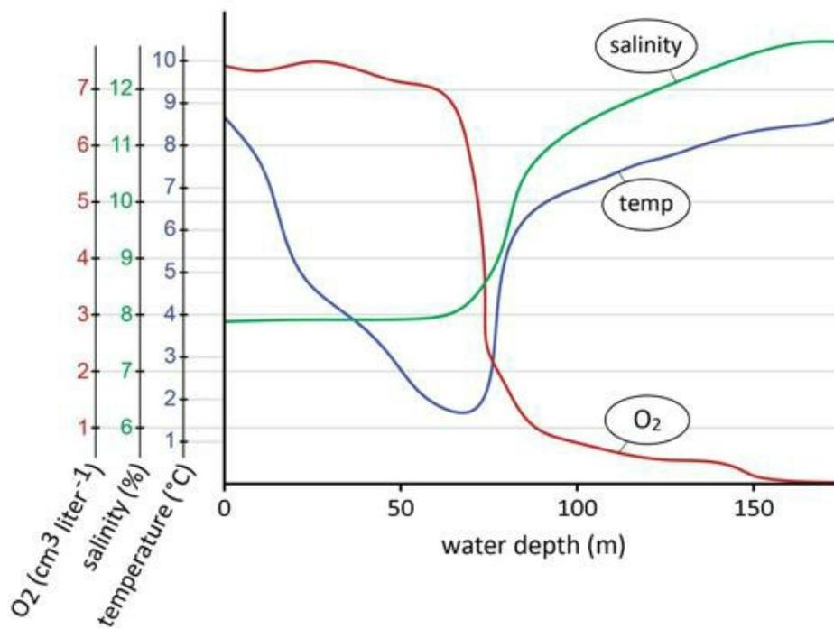
**Fig. 16.5** Vertical profiles in the ocean.<sup>2</sup> Temperature, dissolved oxygen, and salinity profiles, measured at Baltic Sea station, 26 May, 1979.
