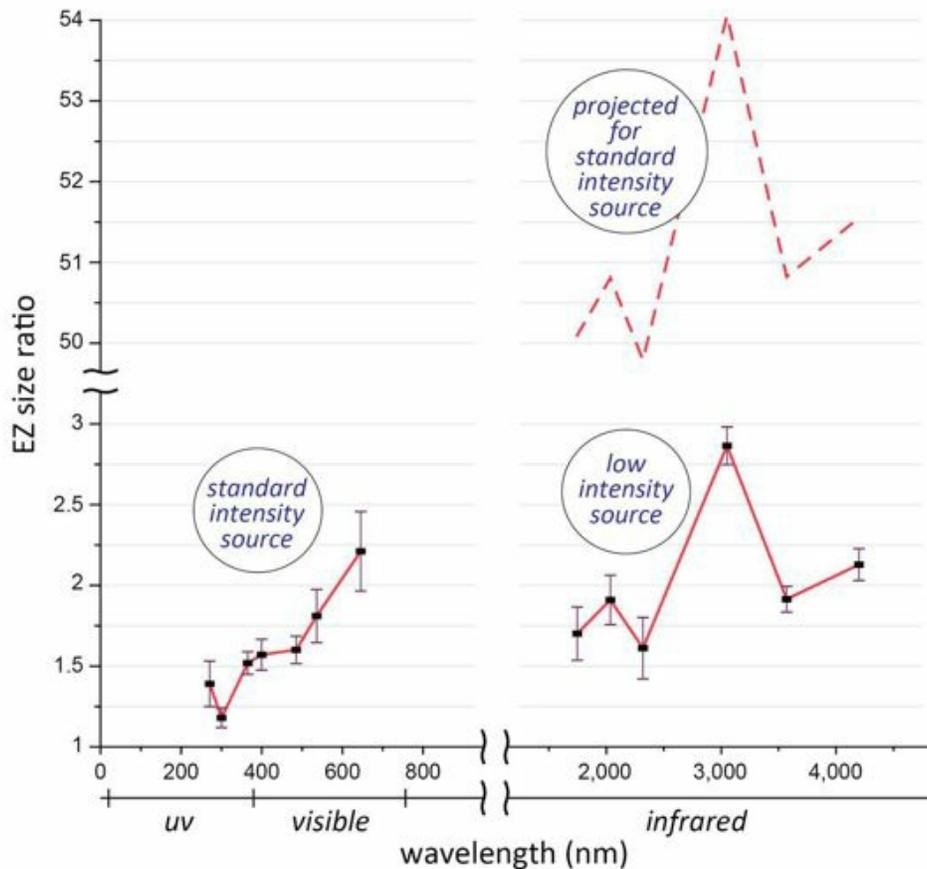
**Fig. 6.2** Effect of incident light wavelength on EZ growth. EZ size ratio (ordinate) refers to EZ size at the end of a five-minute exposure to light, relative to its size before adding light. For technical reasons, data on the right side were obtained with low-intensity light sources. Intensities similar to those used for obtaining the data on the left would have elevated the graph, as estimated by the dashed curve above.
