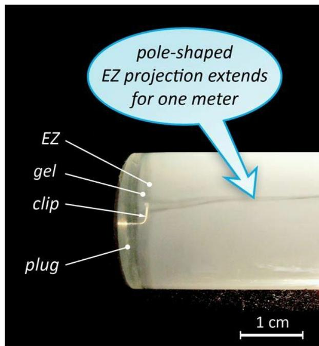
**Fig. 3.8** *Long EZ projection. The disc-like gel creates a disc-like EZ that wedges into a long pole-like projection. The projection can extend at least one meter.*
