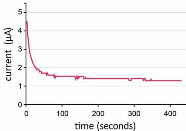
**Fig. 5.7** *Current flow from separated charges in EZ and the water beyond. Current begins flowing immediately after immersing electrodes, maintaining a nonzero plateau value for an extended period of time.*
