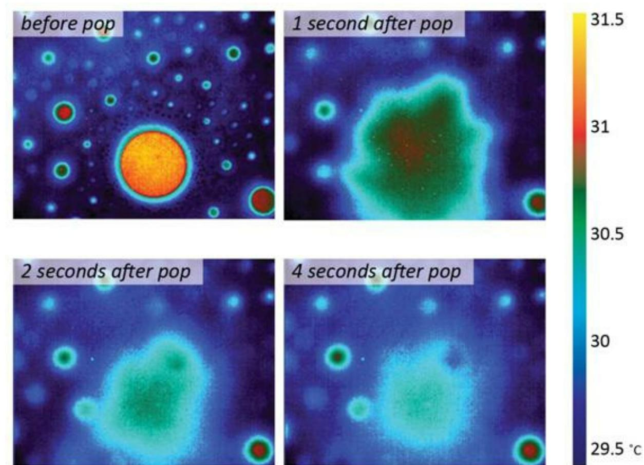
**Fig. 14.7** Bubble collapse. Similar to Figure 14.6, except that one bubble pops spontaneously. Note the dispersal of the zone of high radiant energy. Scale in °C.
