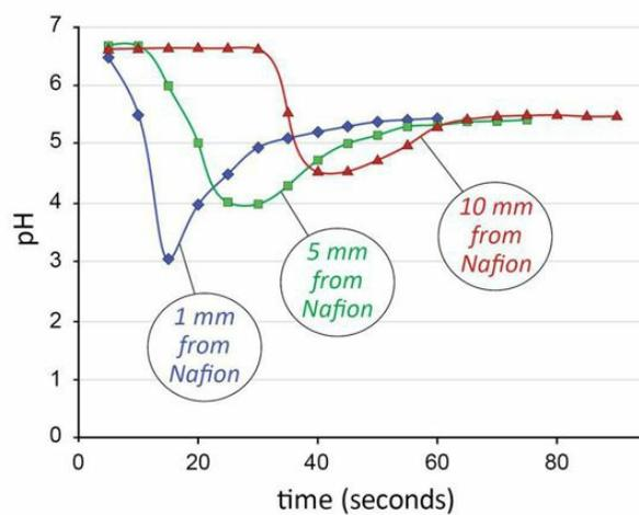
**Fig. 5.1** Time course of pH change following the addition of water to a sheet of Nafion. We measured the pH at three points, as indicated. The pattern suggests a progressively rising wave of protons.
