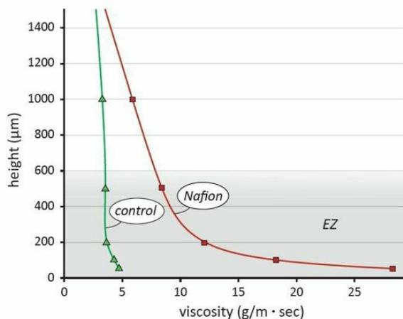
**Fig. 3.17** Viscous character of the EZ (shaded). We measured viscosity in water at various heights above a Nafion surface (red curve). Control (green curve) was obtained with a surface exhibiting little or no exclusion zone.
