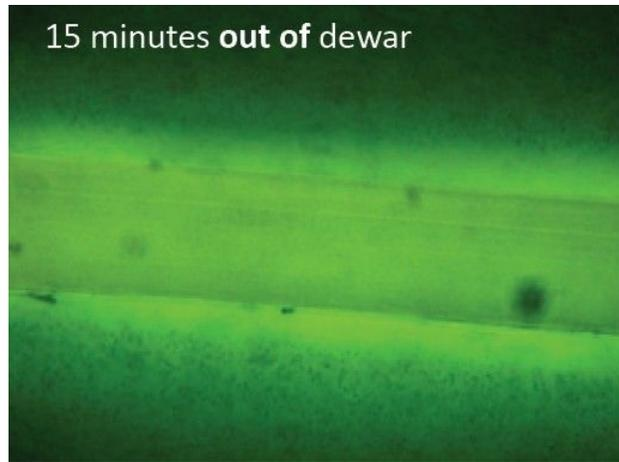
**Fig. 6.3** Reducing incident infrared energy diminishes EZ size. Extracting the chamber returns the EZ size to its original value.
