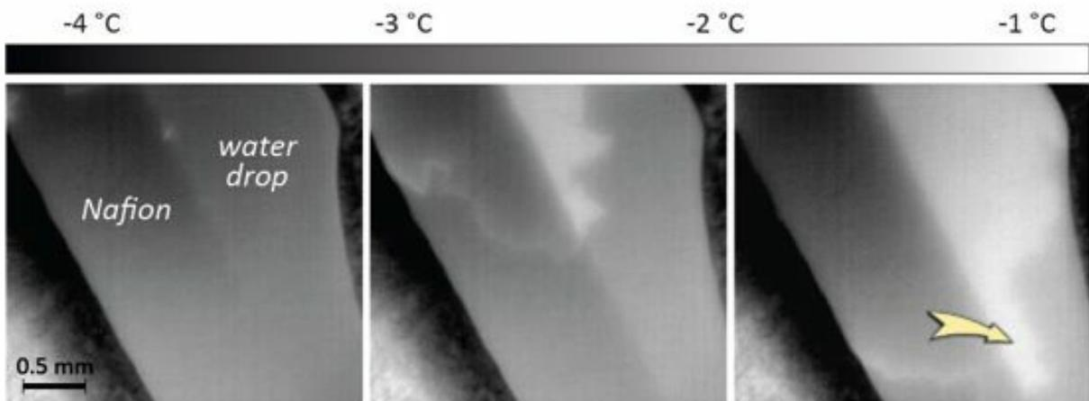
**Fig. 17.3** Sequential progression of droplet freezing on a cold plate, as recorded by an infrared camera. The droplet sits beside a strip of Nafion. Region of freezing begins in the EZ next to Nafion (left, white dot) and tends to propagate most rapidly along the EZ (arrow, right panel).
