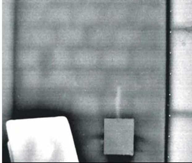
**Fig. 10.5** Interior wall in a room situated just off a corridor. Observed with visible light (top) and with IR light (bottom).<sup>1</sup> The IR image reveals details of the wall's internal structure.
