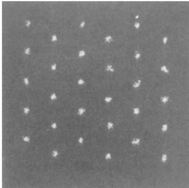
**Fig. 8.3** *Eventual distribution of latex particles: 0.4  $\mu\text{m}$  in diameter, 2% concentration in aqueous suspension.*<sup>3</sup>
