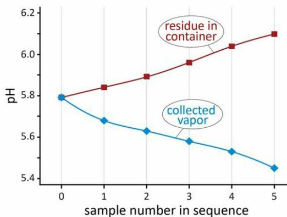
**Fig. 14.5** Results of boiling experiments. Blue curve indicates pH of the vapor, collected after various durations of time. Red curve indicates pH of water remaining in the container following boiling.
