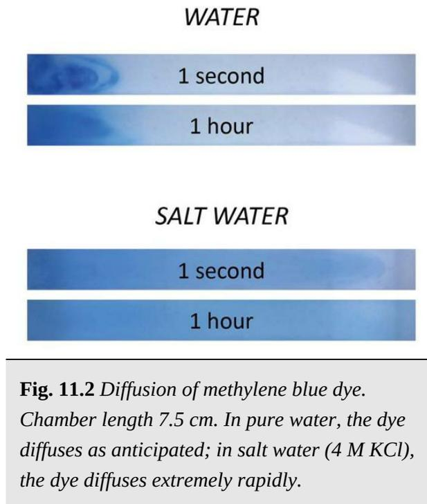
**Fig. 11.2** Diffusion of methylene blue dye. Chamber length 7.5 cm. In pure water, the dye diffuses as anticipated; in salt water (4 M KCl), the dye diffuses extremely rapidly.
