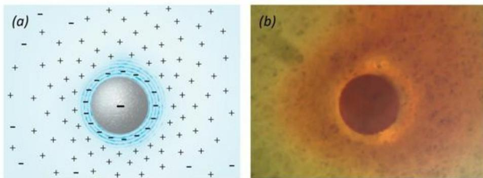
**Fig. 8.9** Spherical particles immersed in water. (a) Diagram showing surrounding charges. (b) Negatively charged bead (dark) immersed in water with pH dye. Lighter region around the dark sphere is the EZ, which excludes pH dye. Intensely red region beyond indicates low pH, or high concentration of protons.
