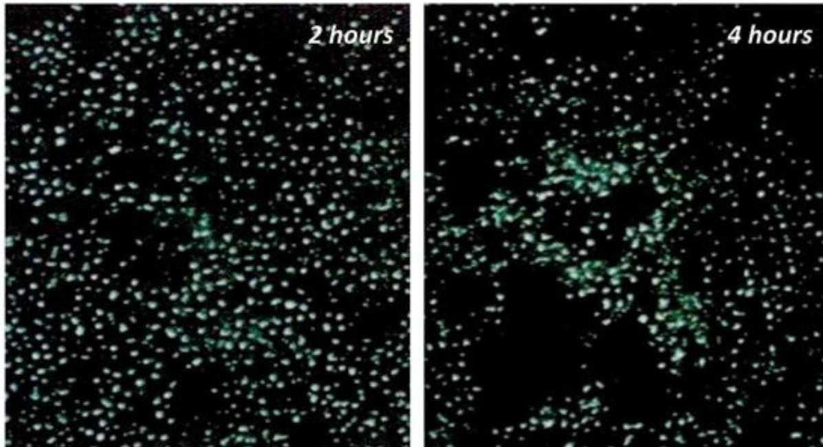
**Fig. 8.4** *Microspheres draw together over time, leaving large voids that contain no microspheres.*
