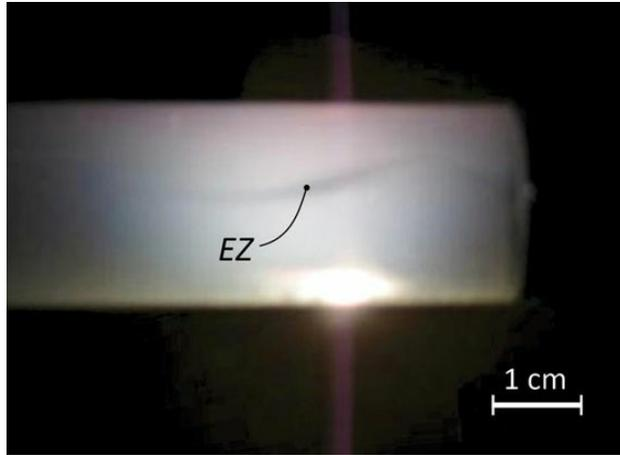
**Fig. 9.13** *Light-induced deflection of microsphere-free zone. This EZ projects from a nucleating surface positioned off to the left. The light beam projects from bottom to top. Microspheres drawn toward the light cause the EZ to shift oppositely.*
