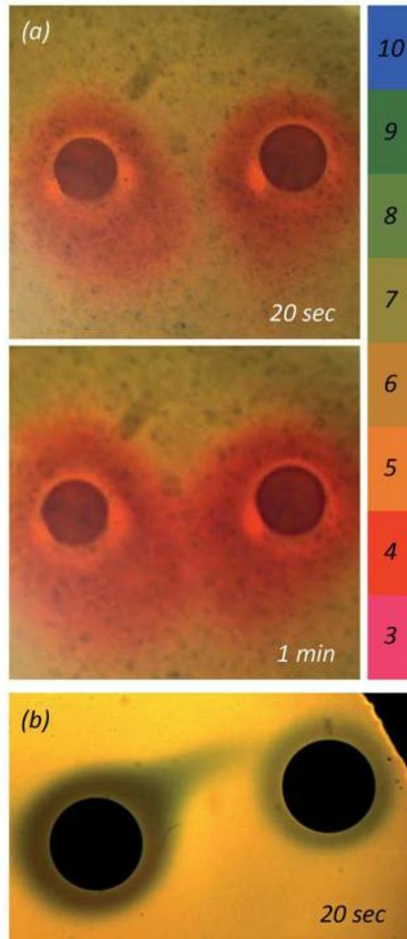
**Fig. 8.11** Unlike charges situated between like-charged spheres. (a) Dye shows region of low pH (numerous protons or hydronium ions) in between two negatively charged beads. At right, pH scale. (b) Region of high pH (negative charges) lying between two positively charged beads. Negative charges sometimes coalesced
