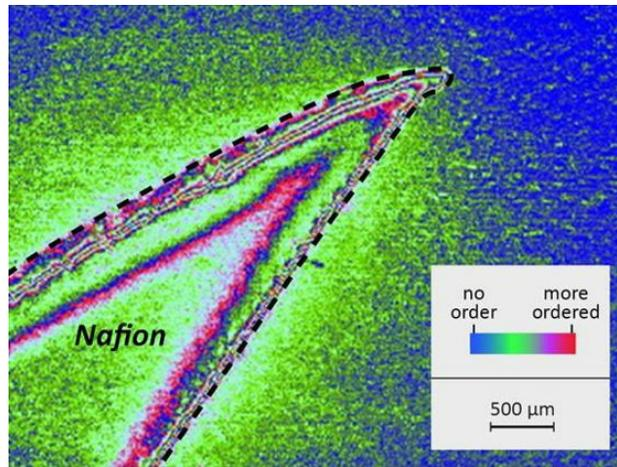
**Fig. 3.20** Arrowhead-shaped piece of Nafion sheet (delineated by broken line) in water, examined using polarizing microscopy. Blue color indicates a random orientation of molecules; red (see scale at right) indicates the highest degree of molecular ordering.
