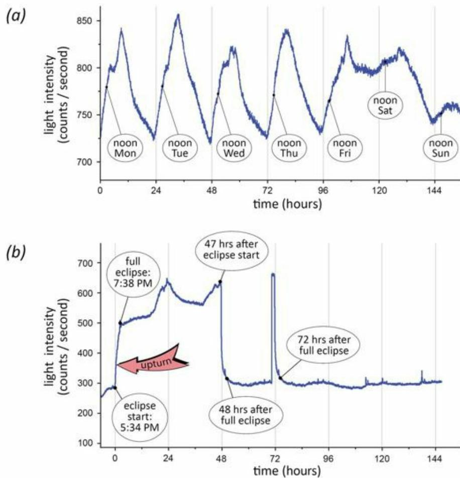
**Fig. 7.3** (a) Light emission recorded from water containing bicarbonate ions and enhanced by dissolved luminol. Note the periodic intensity variation. (b) Similar to (a) but recorded during an eclipse of the moon.
