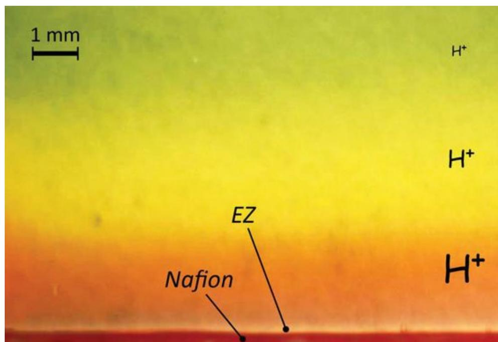
**Fig. 5.3** Proton distribution beyond the exclusion zone (viewing the wide face of a narrow chamber). This image, obtained shortly after pouring water with
