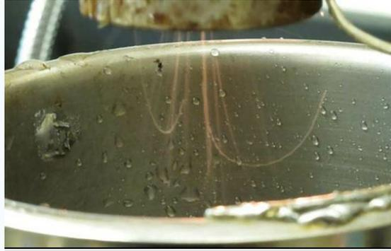
*Droplets falling into the bucket of the Kelvin apparatus, illuminated with red light. When bucket water acquires sufficient charge, falling droplets are repelled upward.*
