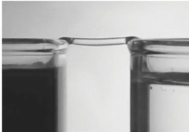
**Fig. 17.16** *Water bridge between two beakers. Bridge has a near-cylindrical cross section that comprises an annulus and a core, which cannot be distinguished in this optical image. Bridge length approximately 3 cm.*
