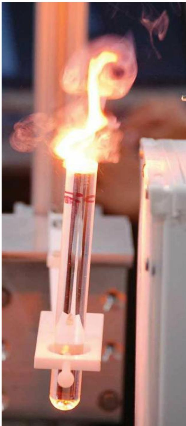
**Fig. 7.6** Salt water exposed to electromagnetic energy. The solution catches fire.<sup>3</sup>
