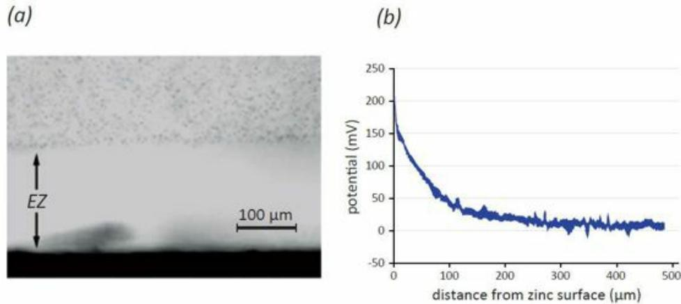
**Fig. 12.9** Zinc-surface features.<sup>4</sup> (a) Exclusion zone found next to zinc. (b) Electrical potential within the EZ
