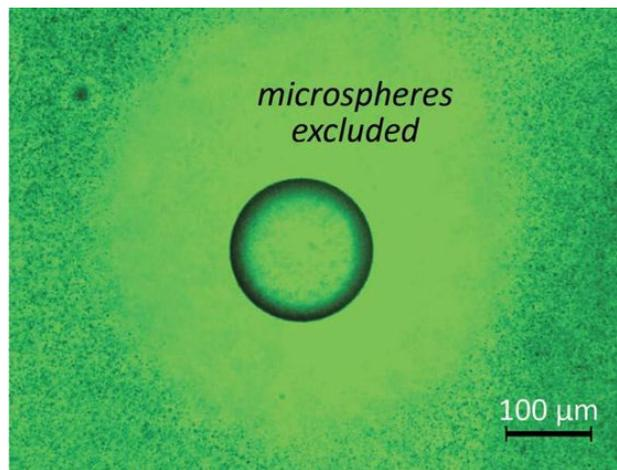
**Fig. 3.7** *Microspheres excluded from the vicinity of a charged gel bead, as seen in an optical microscope. (Color arises because of microscope filter.) We positioned the bead on a glass surface and added the microsphere suspension. The EZ grew with time to the extent shown.*
