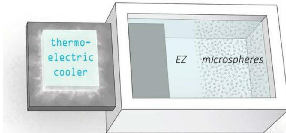
**Fig. 17.4** Cooling apparatus for exploring the relation between EZ and ice formation.
